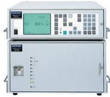
MEXA-1170HCLD Heated Type NOx Analyzer
